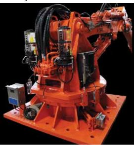
Rotating base assembly incorporates a slewing ring that permits accurate 270° (plus) positioning. Shown with optional auto lube systems.
