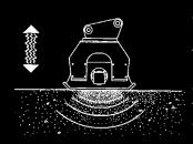
The leader in trench compaction technology, NPK delivers the industry's greatest impulse forces with overall superior performance through hydraulically-operated rotating eccentric action. Greater vibration forces generate stress waves in granular or loose soil material, bringing the soil's air to the surface and packing the particles closer together. Greater impulse action works together with the carrier's downward forces to compact cohesive clay-type soils.
