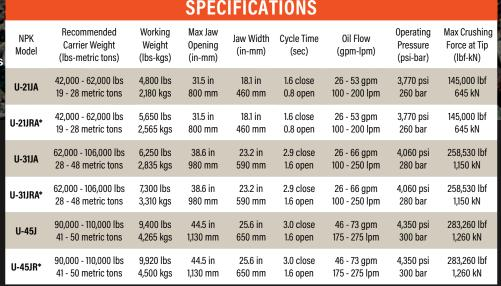
\* "R" models come with full 360° hydraulic rotation for maximum versatility. Working weight includes mounting bracket. Cycle time is full stroke, without material, at maximum oil flow. Specifications subject to change without notice.
