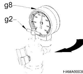
7. Compare the gauge pressure with the “**NITROGEN GAS PRE-CHARGE**” chart in the “**NITROGEN GAS PRESSURE**” section. If the gas is 25 psi (2 bar) or more below the specification, proceed to the “**NITROGEN GAS CHARGING PROCEDURE**” section of the manual. If the pressure is correct, go to the next step.
