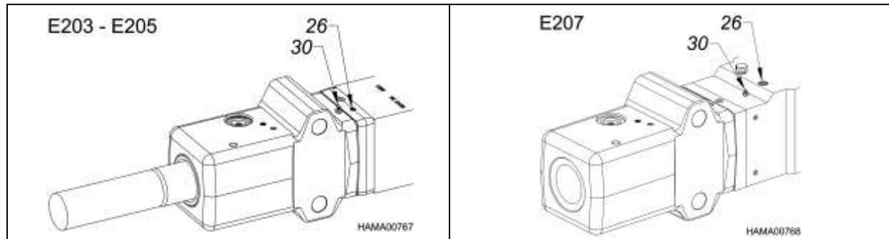
If an Auto Lube System is not used, you can grease the unit manually through the grease fitting (30).
