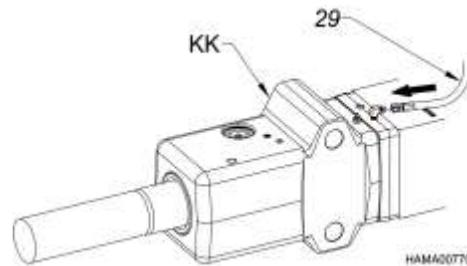
8. Pump twenty more shots of grease, using a grease gun (t37) or power greaser, into the pump assembly (FZ). This will prime the hammer tool cavity and pre-lube the tool (HH). Look for grease coming out around the tool at the tool bushing (see arrow in Fig. 2).
