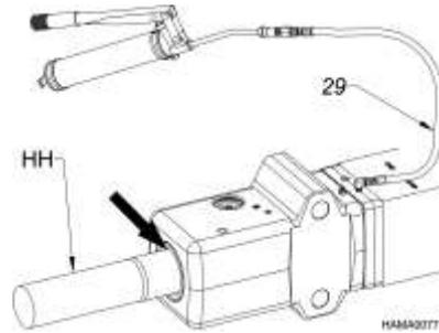
11. Remove the hose fill adapter (a13) and re-connect the grease line (29) to the Auto Lube pump (FZ).
