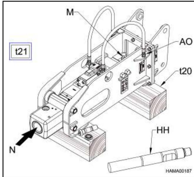
If the NPK HYDRAULIC HAMMER is not to be used for a long period of time (months), it is recommended the gas pressure be discharged at the charge valve (M). The tool (HH) should be removed, and the piston (N) pushed all the way in. Be sure the hydraulic hoses are plugged and grease the exposed end of the piston (N). Grease and reinstall the tool (HH). Cover with a waterproof tarp (t21), not shown.
