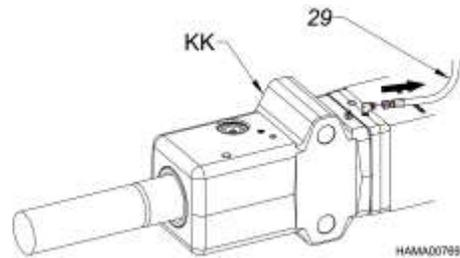
7. Attach a grease gun (t37) or power greaser to the grease line (29) leading to the hammer.
