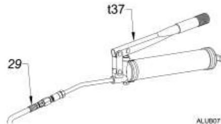
8. Pump grease through the grease line (29) until a steady stream of grease (28) is realized at the opposite (hammer) end.
