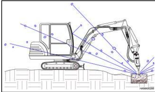
**DO NOT OPERATE THE HAMMER WITHOUT AN IMPACT RESISTANT CAB WINDOW OR SHIELD IN PLACE**
