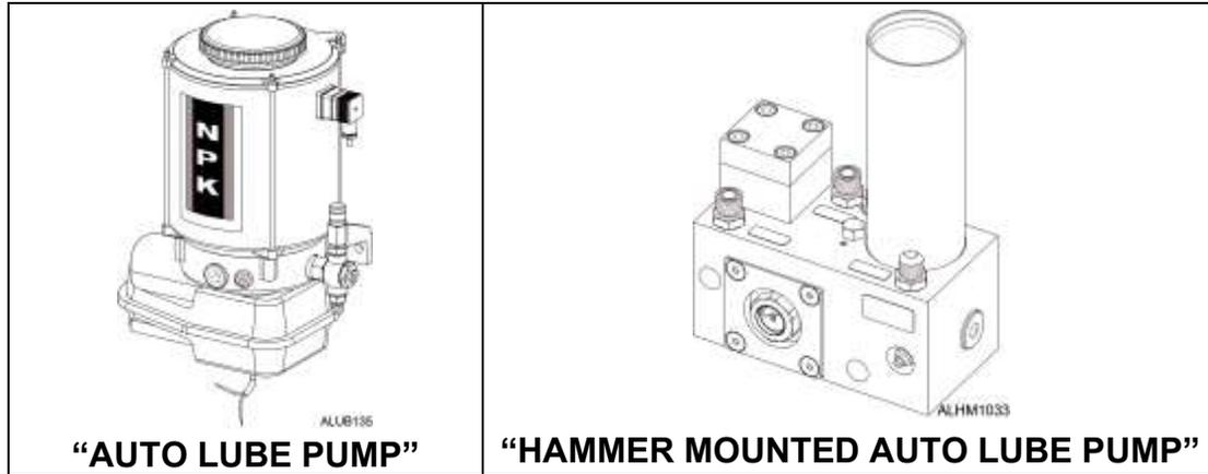
The NPK Auto Lube Systems are designed to automatically provide a continuous supply of grease to the hammer tool and tool bushing, increasing tool and tool bushing life by reducing wear. The Auto Lube pumps are capable of pumping EP2 grease in cold weather. The pump output is adjustable according to the replacements of the hammer model and to compensate for tool bushing wear.
