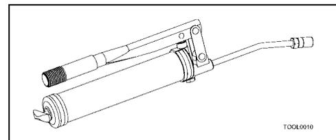
**Second**, if you can't control the grease schedule, such as rental units, then have the operator grease the hammer once every hour of hammer operation. Again, grease the hammer until grease comes out between the tool and tool bushing. This is usually more often than required but is far cheaper than replacing prematurely worn tools and tool bushings.
