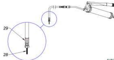
9. Re-attach the grease line (29) to the hammer assembly (KK).
