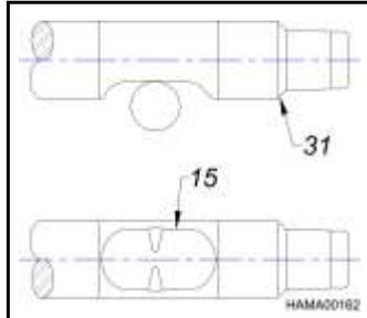
2. Excessive blank hammering will cause chipping (16) in the retaining pin contact area (15). If neglected, the chipping may reduce the life or cause failure of the tool retaining pin. Dress with a grinder.
