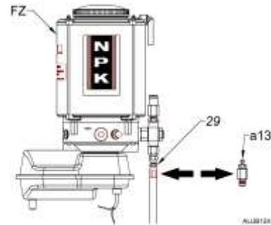
**NOTE:** If the Auto Lube unit has run out of grease, the above procedure should be used to purge all air out of the grease line before using the hammer. Failure to do this will result in an intermittent supply of grease to the hammer.
