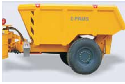
Skip up to 33,000 lbs. (15,000 kg) payload
