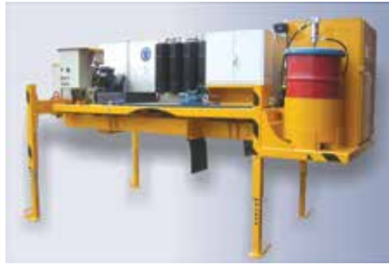
Service Unit: different tank capacities for diesel fuel, oils, greases incl. pumps, compressed air
