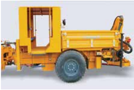
Personnel cabin, crane, loading platform; up to 33,000 lbs. (15,000 kg) payload
