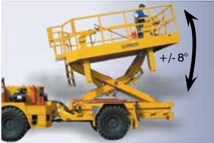
Scissor Platform: up to 8800 lbs. (4000 kg) payload, platform height 11 ft. 6 in. (3500 mm) or higher
