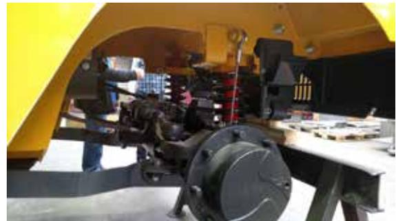
The mine-duty MinCa 5.1 is built on a robust, rigid frame with an innovative, fully independent, heavy-duty coil spring suspension that provides excellent driving comfort and a safe, smooth ride even at higher speeds.
