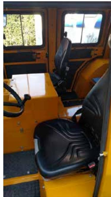
The MinCa 5.1 diesel engine operates with a hydrostatic drive. This transport vehicle has a permanent four wheel drive system with hydraulic steering at the front axle.
