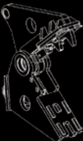
G Jaw Set (Pulverizing) Replaceable Tooth Plate
