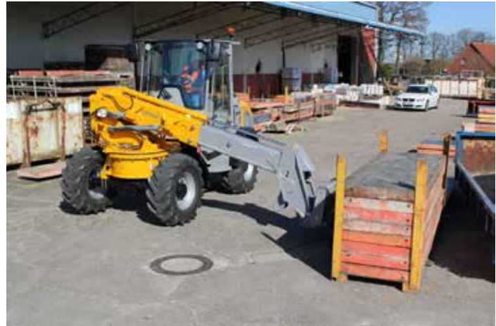
A pivoting boom of ( \pm 90^\circ ) allows for maneuverability in narrow vein mining conditions
