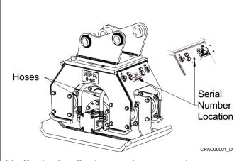
Verify hydraulic hoses between the motor and manifold are tight.
