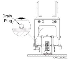
Place compactor on level flat surface. Remove drain plug, oil should be touching the bottom of drain port.
