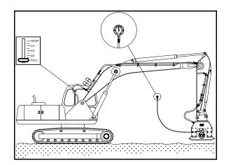
3. Refer to the chart below for the correct relief pressure setting of the compactor model tested. To adjust the relief, use an 11/16" combination wrench to loosen the jam nut and a 5/32" Allen wrench to adjust the relief screw.
