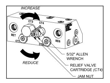
\*Turn adjusting screw in to increase relief setting and turn out (counterclockwise) to reduce relief setting (clockwise).
