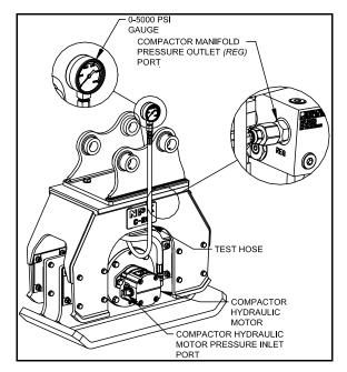
2. Start the machine, run machine at full rpm, activate the compactor circuit. The reading on the gauge will indicate the manifold relief setting.
